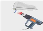
The second way: warm up glutinous gun with glue rod for gluing of plastics. Apply a small amount of glue on dead end of the highway and give to harden it.
